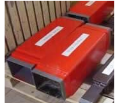
Figure 6.6 : Damper (RHS 260x160x7mm)
