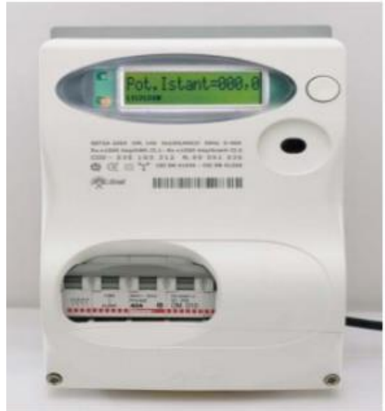
Figure 39 : Smart meter Enel Source : (Vandromme, Dany. 2015)
